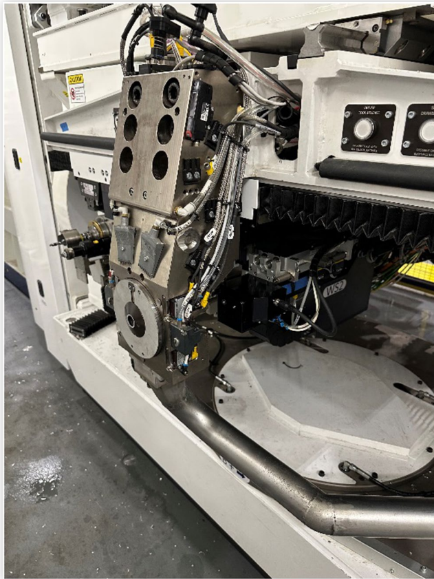
FIGURE 2 Skin side riveting process with BUCA headstone
